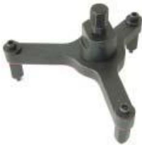
To divide Crank Case and to draw out Crank Shaft.
