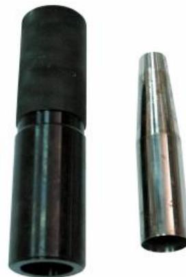
Assemble Oil Seal on Crank Shaft and Avoid Oil Seal Inner diameter Damaged by Crank Shaft Teeth.
