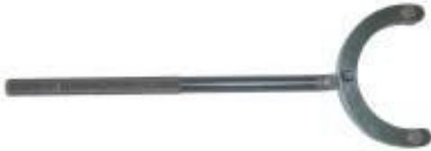
To remove Driven Pulley Assy and Flywheel magneto.
